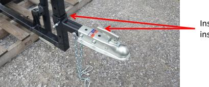
Install Coupler Assembly and insert a Bent Pin and clip.
