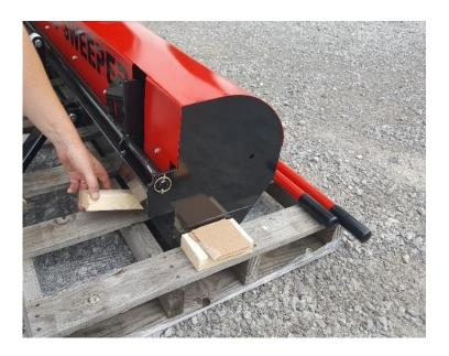
Remove the wooden blocks that are attached to the pallet from the ends and back of the sweeper.
