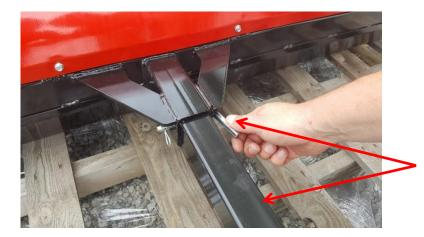
Install Steel Tongue and insert a Bent Pin and clip.
