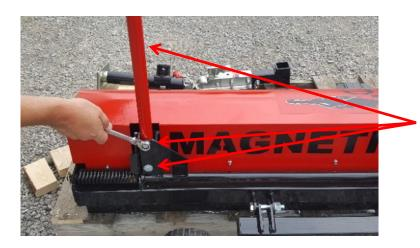
Install Release Handles on each end of the sweeper and tighten using a 9/16 wrench.
