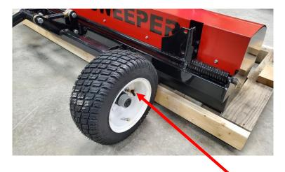
Install both wheels with valve stem facing out.
